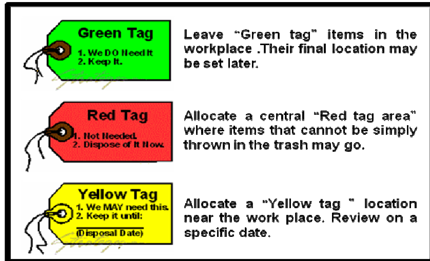
Figure 2.11.Sorting by use of red, yellow and green tags. Adapted from “Toyota production system and lean management,” by PTU’s Gian Jyoti School of TQM & Entrepreneurship, 2010, p.99.
